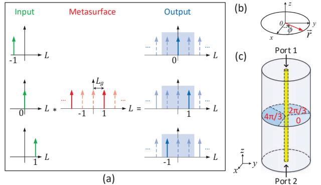
Fig. 3. (a) The  $L$ -space operation of a metasurface featuring the circulation of three modes with SAMs of -1, 0, 1. (b) SAM of a EM wave propagating along the  $+z$ -direction. (c) An ideal model designed to prove the concept of  $L$ -space mode circulation.
