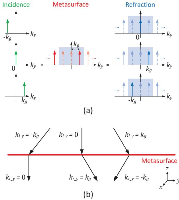
Fig. 2. (a) The  $k$ -space operation of a metasurface showing the circulation of three diffraction modes. Arrows with solid line represent diffraction modes with non-zero amplitude, while arrows with dashed line represent diffraction modes with zero amplitude. (b) A schematic diagram of a transmitting metasurface upon different incoming plane waves as shown in (a).
